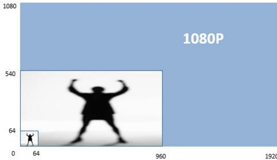
For example, the target in picture below is too large to detect, the man almost covers the whole scene. We suggest adjusting the angle higher so that IP camera can start detecting from a longer distance.
