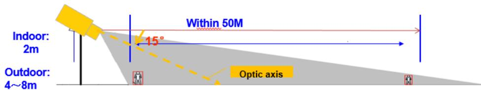
Camera is recommended to be installed 2-3 meters high in doors. If it is installed outside, it should be 3-8m high. If there is fence, the installation height must be higher than the fence.
